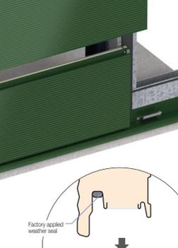
h Apply an unbroken 6mm Ø bead of gun-grade sealant to provide an air seal between back of panel and drip support angle. This air seal should meet the previously installed bubble gasket
