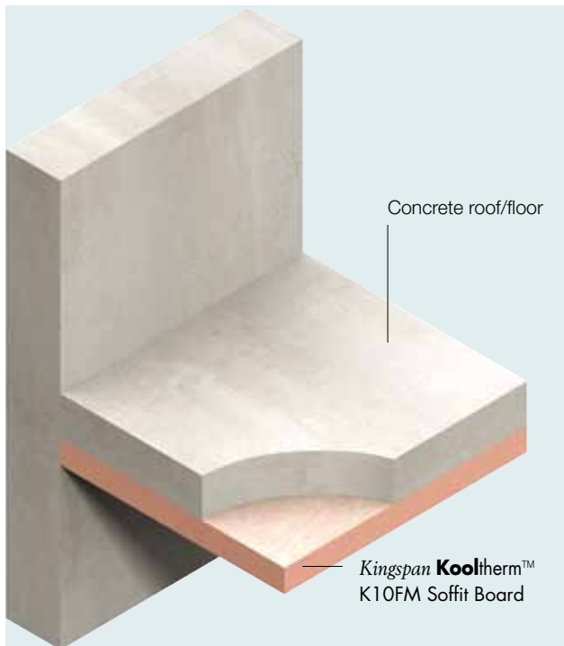
Figure 1 Concrete soffit floor installation
