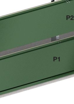
h Install main fasteners through the male joint at each panel end into vertical rail location
